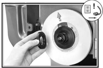
Figure 24. Exposing wheel retaining washer.
